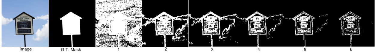
Figure 3.6: Visualization of DCT coefficients for each recompression for a repeatedly compressed image under QF 80. The number below shows recompression counts. Black pixels indicate unaltered DCT coefficients. White pixels indicate the unstable region where DCT coefficients change after compression, which gradually focus on the tampered region as the count increases.
